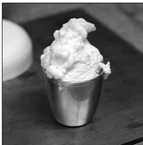
Figure 6-5. Partially reacted reagents overflowing a crucible because of rapid water and carbon dioxide evolution. This can cause loss of sample or contamination. Weight-loss measurements can help detect such losses.
